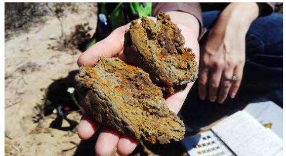
Photo 46: Wetland 6 – Soil sample (30 – 40 cm). Note the mottles.
