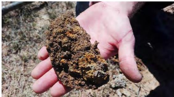
Photo 45: Wetland 6 – Soil sample (0 – 10 cm). Note the mottles.
